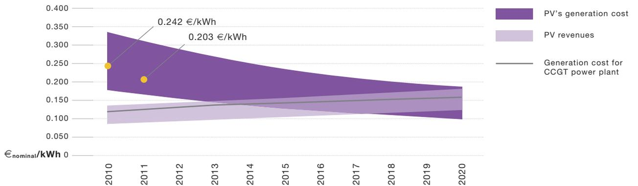
Figure 12C - Dynamic grid parity for industrial PV systems in Europe and generation value competitiveness (comparison with CCGT power plant)
