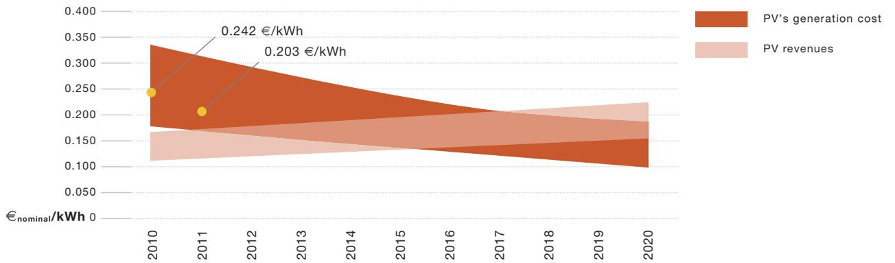
Figure 12B - Dynamic grid parity for commercial PV systems in Europe
